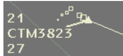
Figure 1 : the ODS comet of an evolving aircraft, the image exhibits direction and acceleration changes
