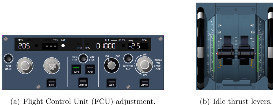
Figure 5. Autoflight and thrust levers setting for the simulation tests.
