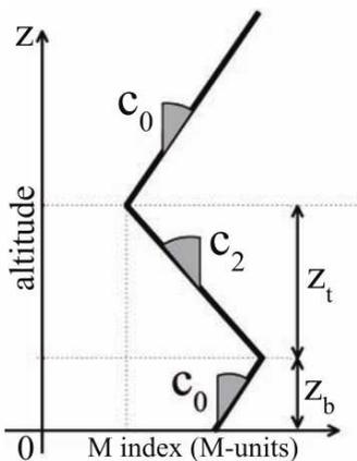
Fig. 5: Trilinear model of the atmosphere.
