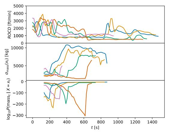
Fig. 9 For the B738, the five trajectories in the test set with the lowest  $P(Y = mass_t | X = x_t)$  are plotted.
