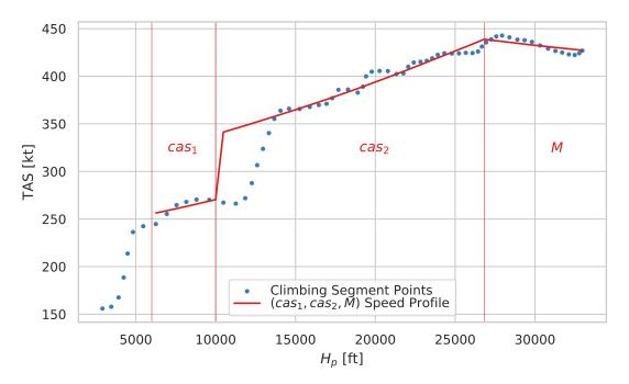
**Fig. 3** A climbing segment and the fitted (*cas*<sub>1</sub>, *cas*<sub>2</sub>, *M*) speed profile. This figure is reprinted from [29] with permission from Elsevier.
