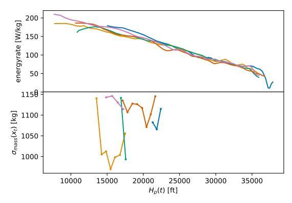
Fig. 7 For the B738, the five trajectories in the test set with the lowest  $\sigma_{mass}$  are plotted.
