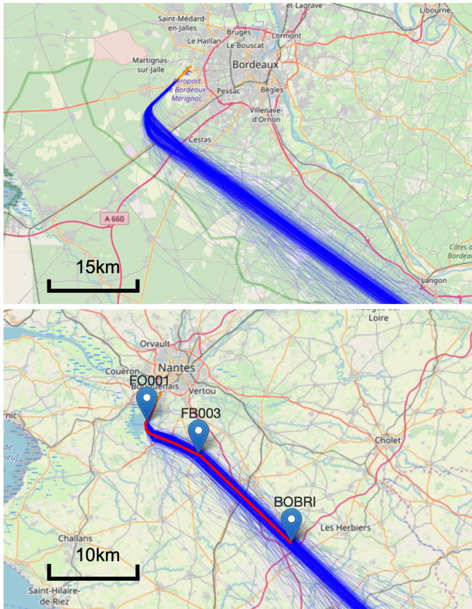
Fig. 6: This figure illustrates the departure procedure deformation. On top, the original trajectories at Bordeaux Airport are represented. At the bottom, the modified trajectories at Nantes Airport. In addition, the expected procedure following different aeronautical way points is shown in red.
