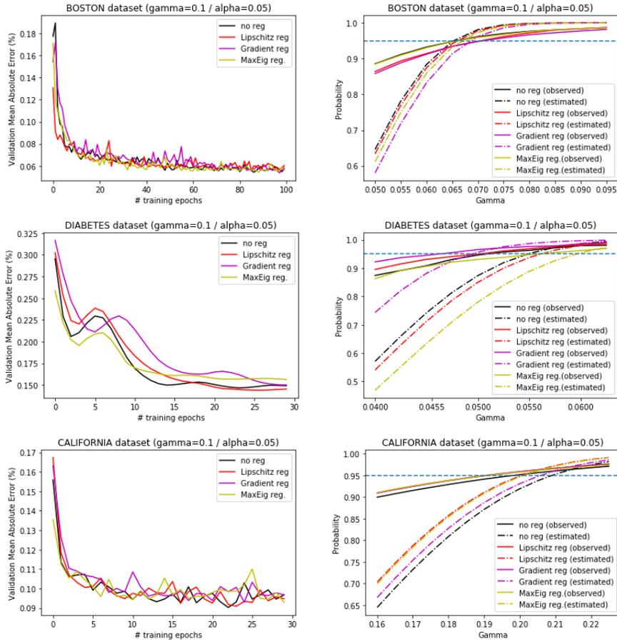
Figure 1: Mean absolute validation error profiles during training (left) & Comparison of  $\mathbb{P}_{\epsilon \sim D} (\|y - y_\epsilon\| \leq \Gamma)$  and exponential tail bound for various levels of  $\Gamma$  (right)
