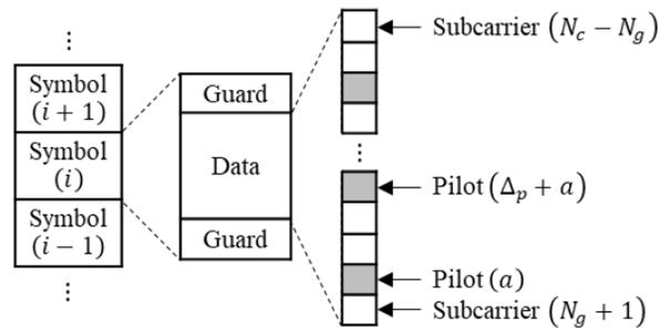
**Figure 1.** OFDM signal structure and pilot inclusion
