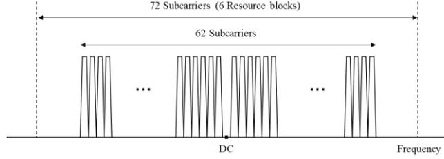
**Figure 4.** LTE PSS and SSS frequency allocation
