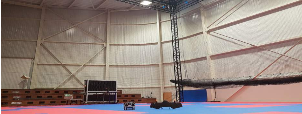
Fig. 15 Dark0 Tail Sitter MAV at rest in the ENAC's flying arena showing two of sixteen Optitrack cameras in the top and the WindShape wind generator in the background.
