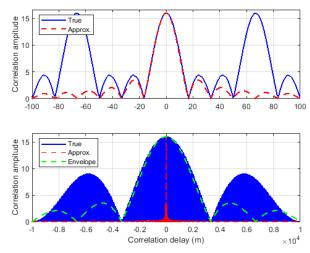
**Figure 10.** True and approximate PCFICH autocorrelation amplitude as a function of the correlation delay for a number of resource blocks equal to hundred; for (top) small correlation delay and (bottom) large correlation delay
