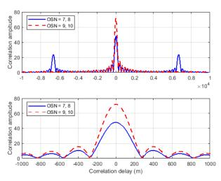
**Figure 5.** PBCH autocorrelation amplitude as a function of the correlation delay for PBCH in OSN 7-10; (top) zoom out (bottom) zoom in
