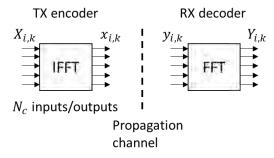
**Figure 1.** OFDM encoding and decoding blocks. Notation:  $X_{i,k}$ , TX data symbols;  $x_{i,k}$ , TX OFDM symbols;  $y_{i,k}$ , RX OFDM symbols;  $Y_{i,k}$ , RX data symbols. The letters i and k represent the OFDM symbol index and the subcarrier index, respectively. Abbreviations: TX, transmitter; RX, receiver
