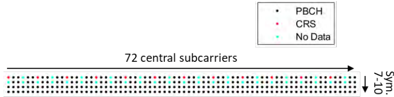
Figure 4. An example of data symbols allocated within the central 72 resource elements of the system bandwidth to antenna port number zero with two antenna ports configuration
