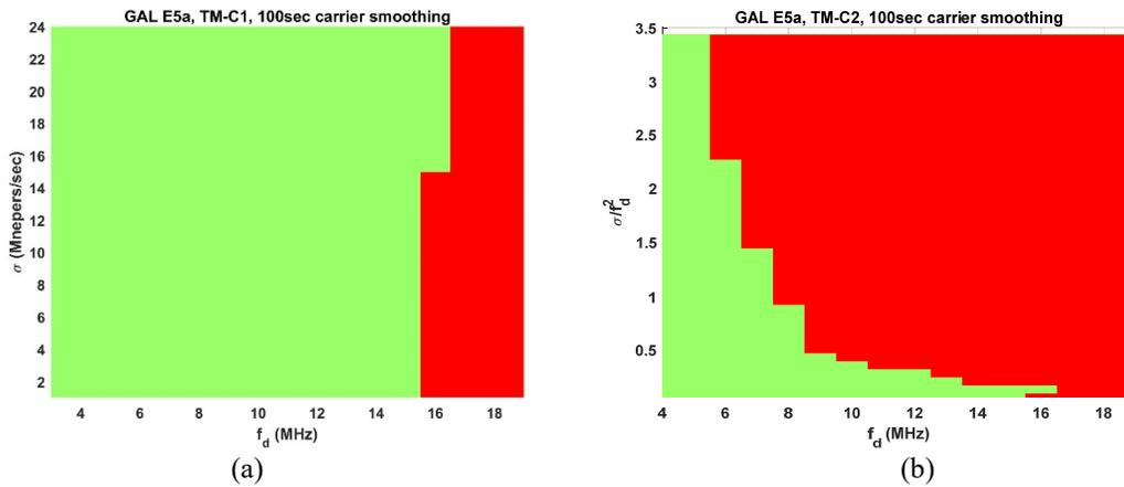
*Fig. 13-Noncompliant region in the threat space for Galileo E5a: (a) TMC1, 100-second time constant and (b) TMC2, 100-second time constant*
