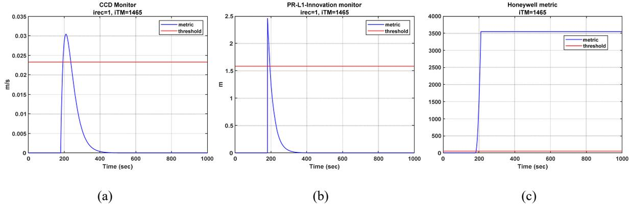
Fig. 11-Time history of (a) the CCD monitor, (b) the DF1-Innovation monitor and (c) Honeywell monitor for the TM C1 type fault ( $\Delta = -0.1$  chip,  $f_d = 1$  MHz and  $\sigma = 23.8$  Mnepers/second), Galileo E1c signal. The red line indicates the threshold.
