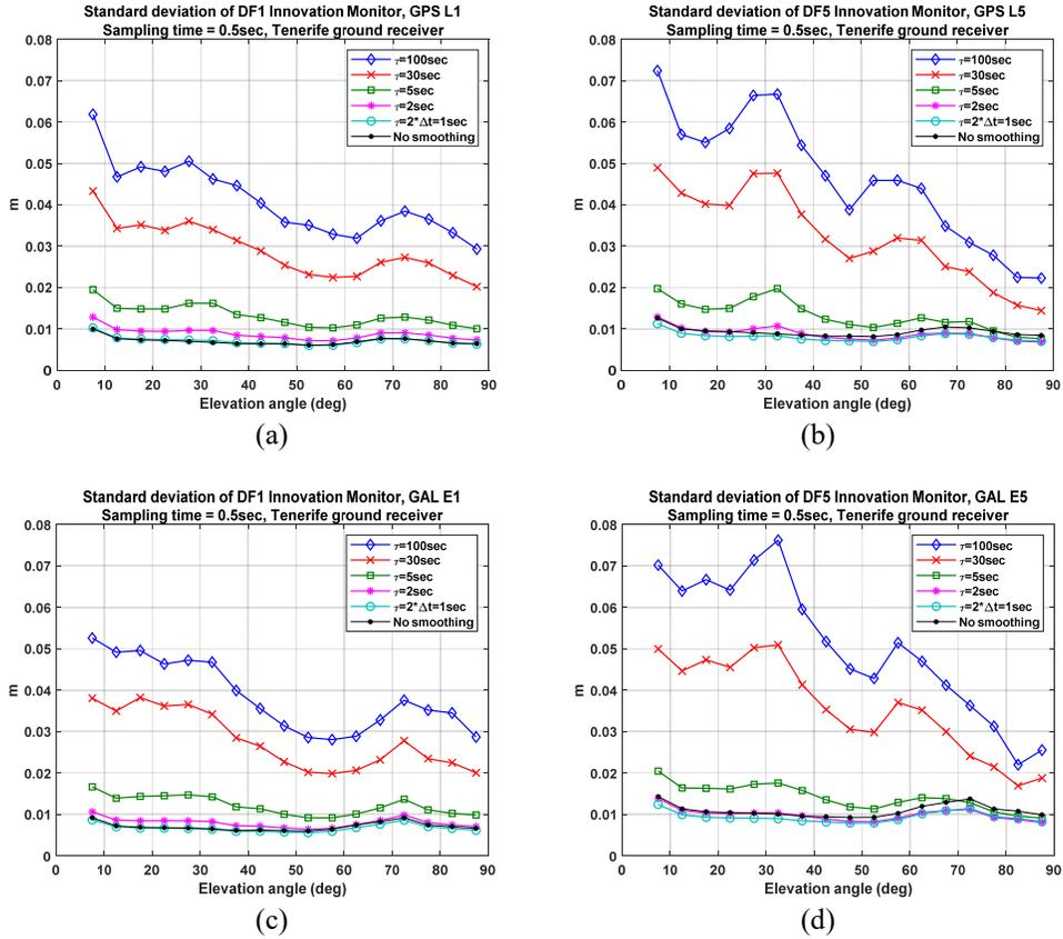
Fig. 4-The standard deviation of the DF-Innovation monitor for (a) GPS L1, (b) GPS L5, (c) Galileo E1 and (d) Galileo E5 signals at Tenerife ground receiver
