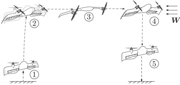
**Figure 1.** Typical flight phases of micro air vehicles with transitioning flight capabilities: 1 – Vertical take-off; 2 – Transition; 3 – Forward flight; 4 – Hover flight; 5 – Vertical landing. The vector  $W$  represents the wind disturbances.
