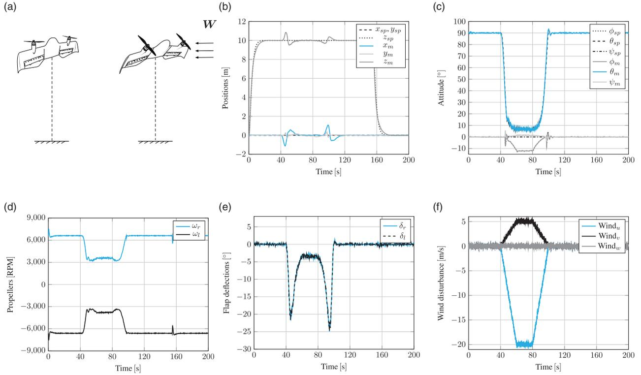
**Figure 10. (#Flight 1)** – Vertical take-off and transition flight to assure position tracking during high crosswind. On the top, from left to right: simulation illustration, positions in the inertial coordinate frame and attitude. On the bottom: propeller speeds ( $\omega_l < 0$  and  $\omega_r > 0$ ) due to counter-rotation sense, flap deflections ( $\delta_l$  and  $\delta_r$ ) convention negative for pitch-up, and wind disturbance.
