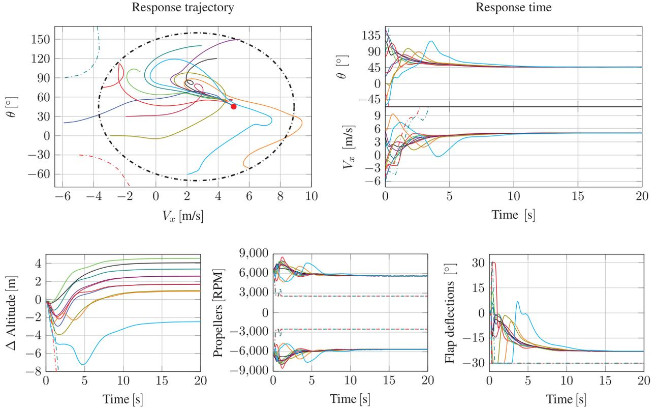
**Figure 12.** Initial pitch angle and forward speed condition analysis during the transitioning flight phase without wind disturbances. Forward speed setpoint equals to 5 m/s, the MFC architecture computes the pitch angle setpoint approximately equals to  $45^\circ$ .
