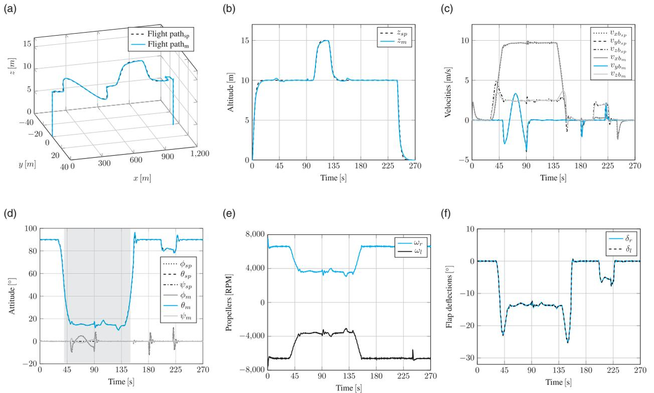
**Figure 16.** (#Flight 3) – Entire flight envelope simulation in relatively calm flight conditions. On the top, from left to right: the 3D flight path, altitude and velocities in the body coordinate system. On the bottom: attitude, propeller speeds and flap deflections.
