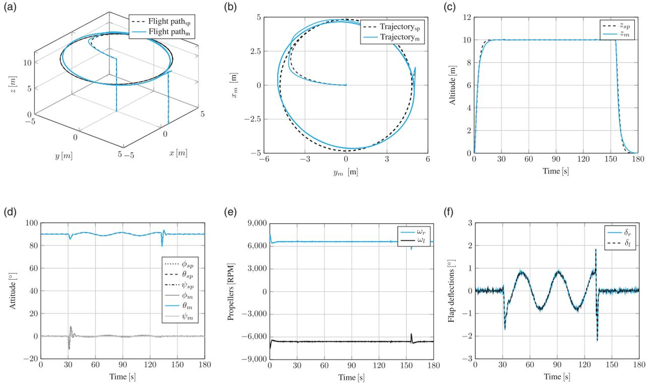
**Figure 11. (#Flight 2)** – Circular position tracking in hover flight mode. On the top, from left to right: the 3D flight path, North and East positions and altitude. On the bottom: attitude, propeller speeds and flap deflections.
