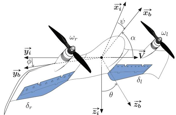
**Figure 4.** Illustration of the used coordinate frames, angles and actuators. The inertial coordinate frame is represented by  $\mathcal{R}_i = \{\vec{x}_i, \vec{y}_i, \vec{z}_i\}$  and the body coordinate frame by  $\mathcal{R}_b = \{\vec{x}_b, \vec{y}_b, \vec{z}_b\}$ .
