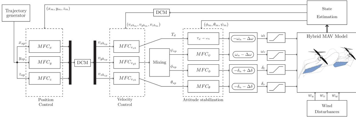
**Figure 6.** Cascaded MFC architecture designed for tailsitter MAVs. Position control blocks send desired velocities for the velocity control blocks that compute the necessary thrust value as well as the references for attitude stabilization control loop. Based on these desired values, propeller speeds ( $\omega_b$ ,  $\omega_r$ ) and flap deflections ( $\delta_l$ ,  $\delta_r$ ) are defined. MAV: micro air vehicle; DCM: Direction Cosines Matrix.
