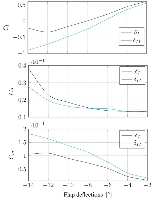
Figure 3. Variation of the sectional lift  $C_l$ , drag  $C_d$ , and moment coefficients  $C_m$  with respect to flap angles for different flap configurations: double-flap ( $\delta_{II}$ ) control surface and a single-flap ( $\delta_I$ ) control surface
