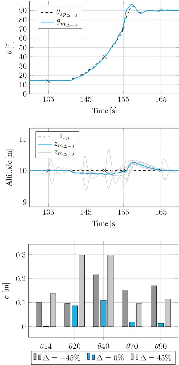
**Figure 13.** Parameter variation analysis for different points in the forward-to-hover transition. The black crosses in altitude and pitch angle trajectories indicate the points in which the parameters were changed.  $\Delta$  represents the variation of nominal mass and inertia in percentage. The standard deviation between the altitude setpoint and its measurements is denoted by  $\sigma$ .
