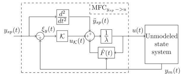
Figure 5. Overview of the model-free control schema.
