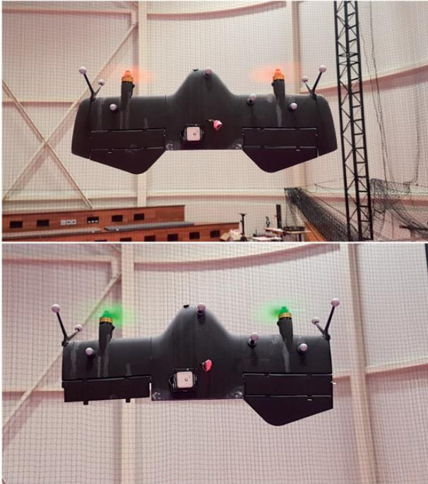
**Figure 21.** Tailsitter MAV configurations used during flight tests. At the top, DarkO with nominal wings, control surfaces and two-blade propellers. At the bottom, DarkO has been modified by removing its wingtips, half of its control surface and three-blade propellers were used.
