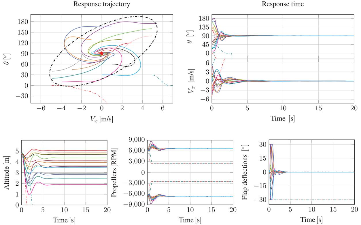
**Figure 7.** Initial pitch angle and forward speed condition analysis during hovering flight phase without wind disturbances. Forward speed setpoint equals to 0 m/s, the MFC architecture computes the pitch angle setpoint equals to  $90^\circ$  in order to reach the stationary flight.
