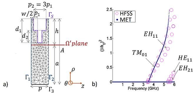
Figure 15: a) Unit cell mesh and dimensions:  $A = 39.3 \text{ mm}$ ,  $a = 23.58 \text{ mm}$ ,  $d_1 = 14.3 \text{ mm}$ ,  $d_2 = 7 \text{ mm}$ ,  $h = 15.72 \text{ mm}$ ,  $p = 10.3 \text{ mm}$ ,  $p_1 = 2.5 \text{ mm}$ ,  $p_2 = 7.5 \text{ mm}$ , and  $w = 5 \text{ mm}$ . b) Dispersion diagrams of the corrugated cylindrical waveguide obtained with MET (dots) and HFSS (circles).
