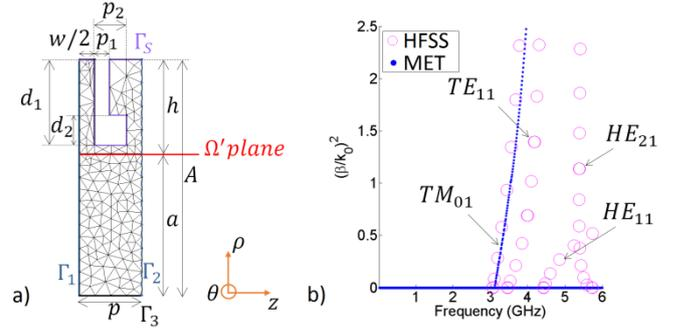
Figure 12: a) Unit cell mesh and dimensions:  $A = 39.3 \text{ mm}$ ,  $a = 23.58 \text{ mm}$ ,  $d_1 = 14.3 \text{ mm}$ ,  $d_2 = 2.5 \text{ mm}$ ,  $h = 15.72 \text{ mm}$ ,  $p = 10.3 \text{ mm}$ ,  $p_1 = 2.5 \text{ mm}$ ,  $p_2 = 5.3 \text{ mm}$ , and  $w = 5 \text{ mm}$ . b) Dispersion diagrams of the corrugated cylindrical waveguide obtained with MET (dots) and HFSS (circles).
