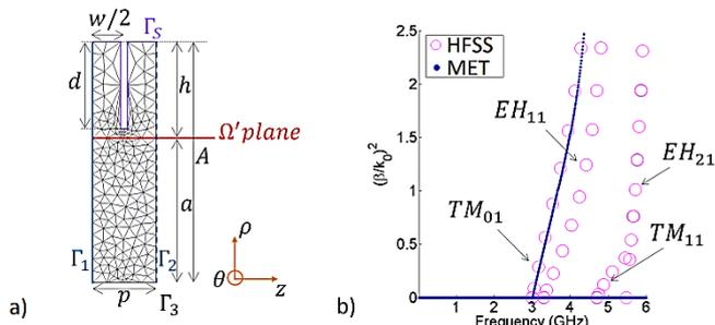
Figure 6: a) Unit cell mesh and dimensions:  $A = 39.3 \text{ mm}$ ,  $a = 23.58 \text{ mm}$ ,  $d = 14.3 \text{ mm}$ ,  $h = 15.72 \text{ mm}$ ,  $p = 10.3 \text{ mm}$ , and  $w = 9.28 \text{ mm}$ . b) Dispersion diagrams of the corrugated cylindrical waveguide obtained with MET (dots) and HFSS (circles).
