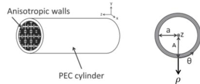
Figure 1: A cylindrical waveguide with anisotropic walls.
