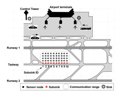
Fig. 1. Deployment of the subnetwork considered in the experiment for an ASAS case.
