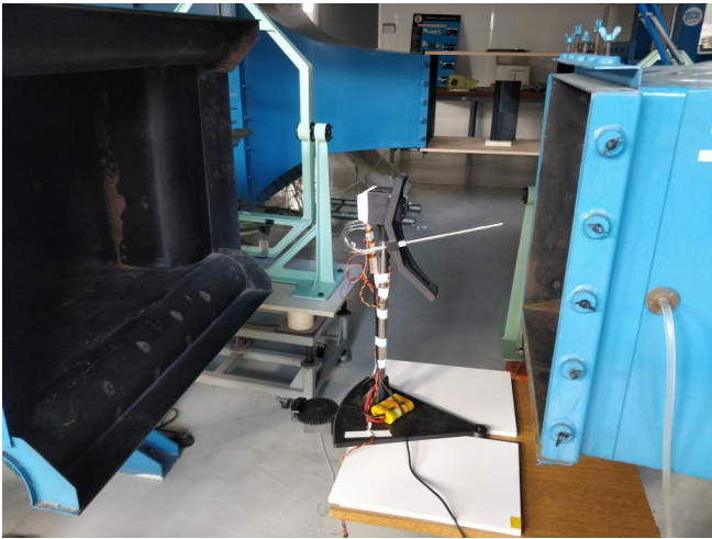
Figure 12: Calibration bench located inside the test section of ENAC's low speed wind-tunnel.
