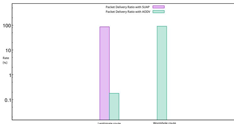
Figure 7 Packet delivery rate in the context of a Wormhole attack
