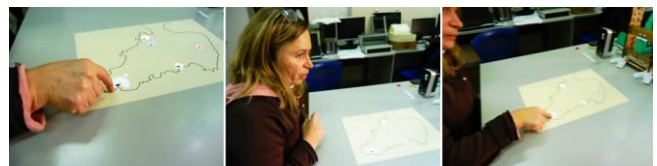
Figure 3. With SAR, the user draws directly on the graphics with the finger (left) and registers the audio feedback (center) in the creation mode. On the exploration mode, the feedback is played when the user touches the zone (right).
