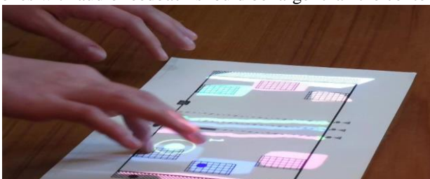
Figure 6. A student explores the Torball tactile graphics. Interactive audio content zones are colored by projection.
