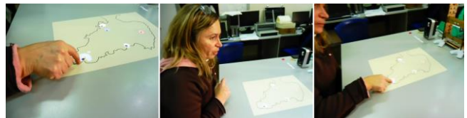
Figure 3. With SAR, the user draws directly on the graphics with the finger (left) and registers the audio feedback (center) in the creation mode. On the exploration mode, the feedback is played when the user touches the zone (right).
