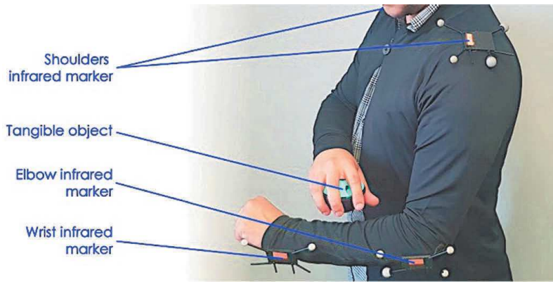
Fig. 2. Placement of the infrared tracking markers
