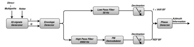
Fig. 2: Block diagram of the VOR receiver.
