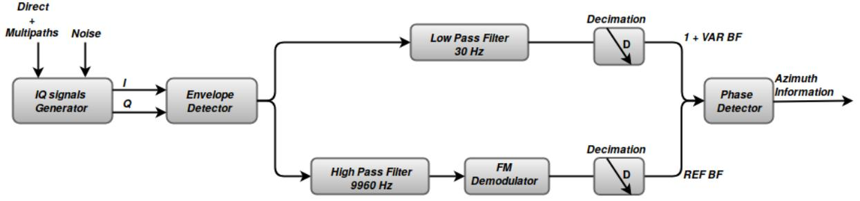
Fig. 2: Block diagram of the VOR receiver.
