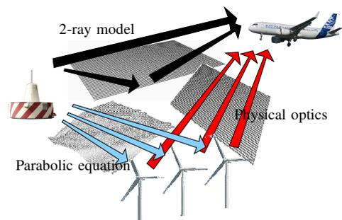
Fig. 1: Overview of the method to compute multipath [3].
