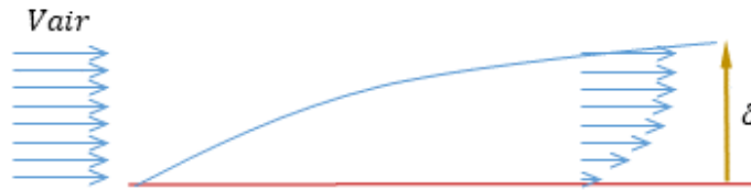
Fig. 18 Boundary layer velocity profile in airplane frame
