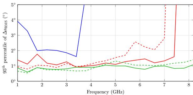
Fig. 5. Simulated (solid line) and measured (dashed line) 95<sup>th</sup> percentile of  $\Delta a_{\text{RMS}}$  obtained from the *Four Season* VA for the estimation of the: (a) vertically- (red line) or (b) horizontally-polarized (green line) EM field using RPC 00. The blue line corresponds to the DoA estimation accuracy of the vertically-polarized EM field achieved from RPC 0.
