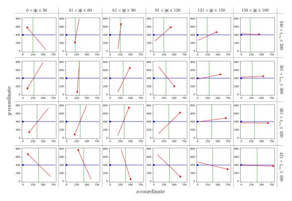
Figure 9. Generated scenarios are classified into 24 groups, based on their time to CPA (t<sub>CPA</sub>, across the rows) and conflict angle ( $\phi$ , across the columns).
