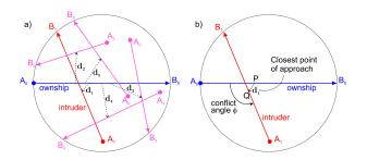
Figure 2. a) Example of a conflict scenario involving a two-aircraft conflict in the presence of four surrounding aircraft.  $A_0B_0$  is the ownship and  $A_1B_1$ is the intruder. b) The conflict pair where **PQ** is the closest distance between two aircraft.
