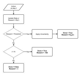
Figure 8. Flowchart to compute reward for each resolution
