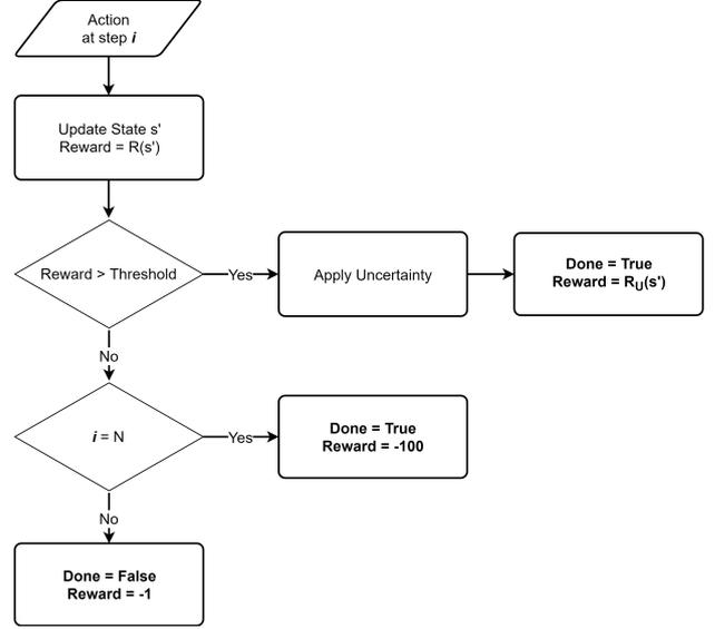
Figure 8. Flowchart to compute reward for each resolution
