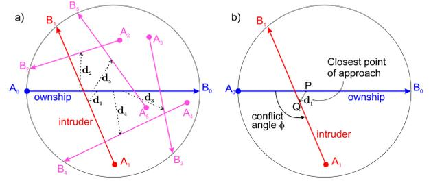
Figure 2. a) Example of a conflict scenario involving a two-aircraft conflict in the presence of four surrounding aircraft.  $\mathbf{A}_0\mathbf{B}_0$  is the ownship and  $\mathbf{A}_1\mathbf{B}_1$  is the intruder. b) The conflict pair where  $\mathbf{PQ}$  is the closest distance between two aircraft.
