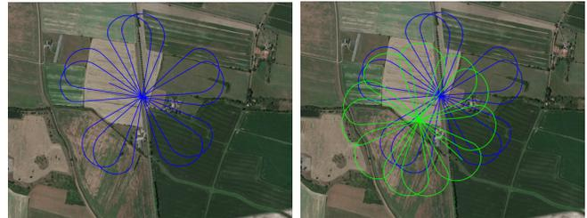
Fig. 8. View in 2D of the KML path of the two UAV using the rosette pattern
