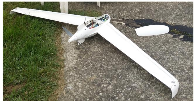
Fig. 11. Picture of the UAV designed for the NEPHELAE project (without the payload)
