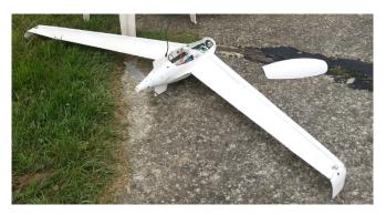
Fig. 11. Picture of the UAV designed for the NEPHELAE project (without the payload)
