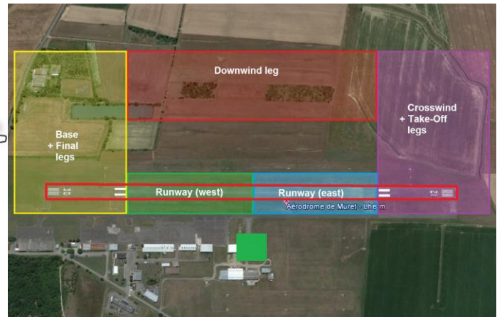
Figure 3. Runway circuit and airport description. On the left, a diagram of a typical runway circuit, which separates the four legs composing an approach segment: crosswind, downwind, final leg and then the runway. On the right, each area is represented on a satellite view of Muret airport. On the two images, the runway is highlighted in red lines, and the position of the control tower is represented with a plain green square.
