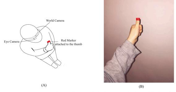
**Fig 8. Finger calibration.** (a) A user performing a calibration using her thumb as a target. A red marker is attached to the tip of her thumb to allow easy detection of her thumb using computer vision techniques. (b) Illustration of a frame obtained in the world camera video stream.
