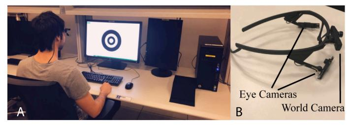
Fig 7. Setup and apparatus. Illustration of (A) the experimental setup and (B) the Pupil Labs eye tracking system. One eye camera was used during the study. https://doi.org/10.1371/journal.pone.0213675.g007
