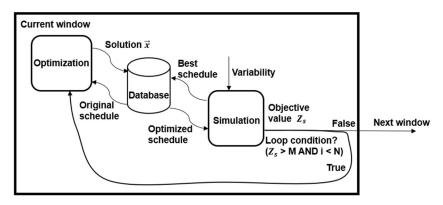
Figure 3: Architecture of the Sim-Opt Loop
