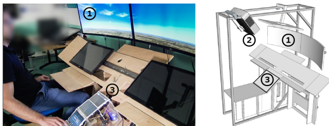
Figure 3. The cockpit platform, (1) 34 inch curved screens, (2) projector, (3) prototype integration area
