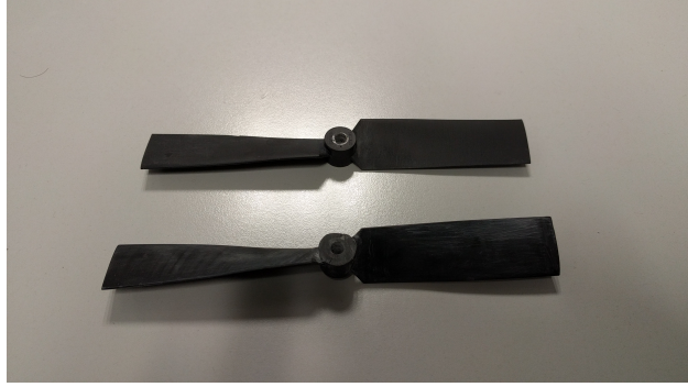
Figure 8: 3D Printed NACA propellers
