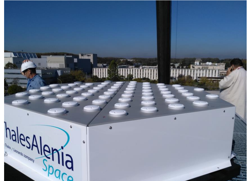
« Innovative » MEOLUT architecture 1 phase array antenna tracks all in view MEO satellites
