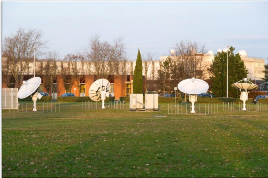
« Classical » MEOLUT architecture 1 dish antenna tracks 1 MEO satellite
