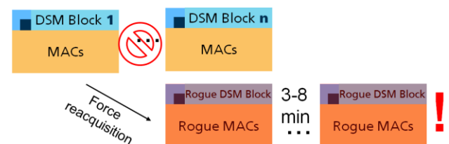
Figure 8 – Schematic representation of a jam and spoof attack.
