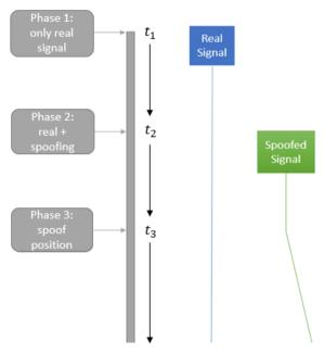
Figure 10 – Spoofing attack steps
