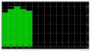
Figure 18 – C/N<sub>0</sub> (in dB) values observed in the COTS receiver with the Intermediate attack
