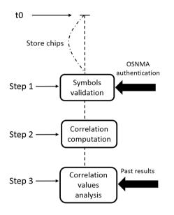
Figure 5 – Anti-replay processing schema
