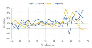
Figure 25 – High-power attack (5dB increase) spoofing correlation variation
