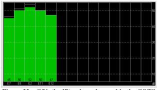
Figure 22 – C/N<sub>0</sub> (in dB) values observed in the COTS receiver with the High power attack
