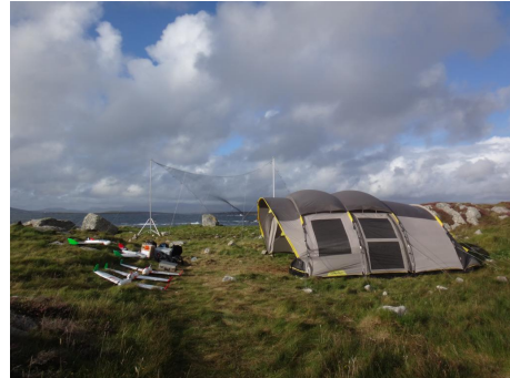
Figure 1: Fleet of UAVs for meteorological studies in harsh and remote location. A net is required to land the planes. Courtesy of Greg Roberts from French Meteorological Research Center.
