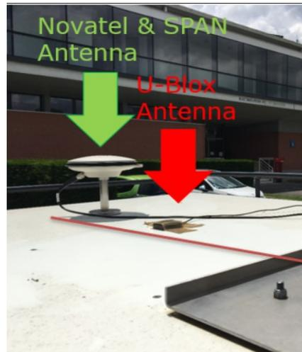
Figure 2b- Rooftop of the vehicle, showing the U-Blox and NovAtel antennas
