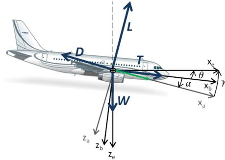
Fig. 1. External Forces on Aircraft During Descent Phase
