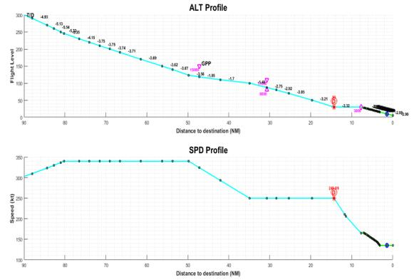
Fig. 15. Flight Trajectory computed by FMS simulator
