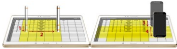
Figure 4: Intersection technique: stack (1) and translation (2) to select columns and stack (3) and translation (4) to select rows.
