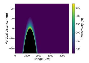
Fig. 1. N index along the propagation scene. Earth is in black.
