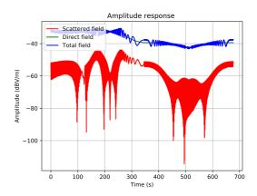
Fig. 3. Electric field (dBV/m) along the aircraft trajectory.
