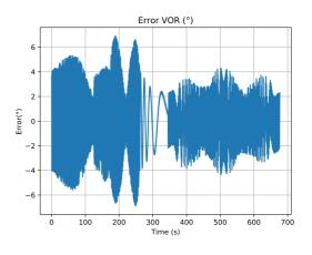
Fig. 5. VOR Error along the trajectory.
