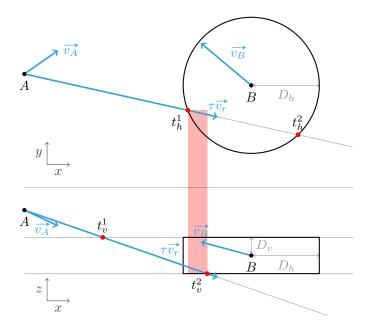
Fig. 1. Horizontal (above) and vertical (below) projections of the geometric model in 4D: a conflict will occur within time  $\tau$  if and only if the relative speed  $\vec{v_r}$  scaled by  $\tau$  crosses the protection volume.
