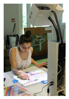
Figure 1. A visually impaired student exploring the multisensory map. The system augments a tactile map with projection and audio output.
