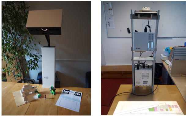
Figure 4. PapART hardware (a) first and (b) second version.
