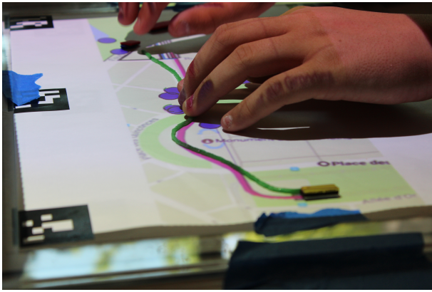
Figure 7. Construction Mode: building a map using Wikki Stix and magnets combined with projection and audio feedback.
