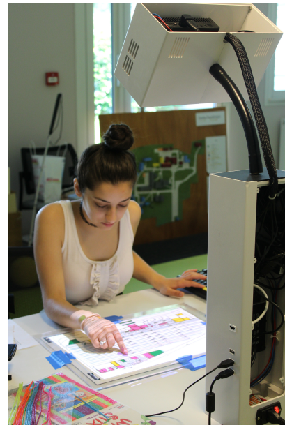
Figure 1. A visually impaired student exploring the multisensory map. The system augments a tactile map with projection and audio output.
