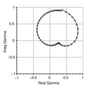
Fig. 11. Real versus imaginary part of the input reflection coefficient (Gamma) of the evolution  $N^{\circ}1$  between 300 MHz and 1.5 GHz. The square points correspond to the simulation values. The full line corresponds to the interpolation with the rational fraction.
