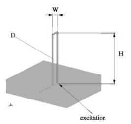
Fig. 7. Basic folded-monopole. H=74mm, W=10mm, D=2mm.
