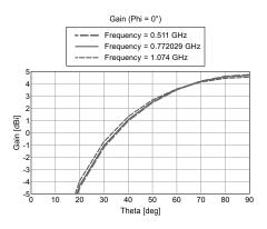
Fig. 21. Cage antenna gain (dBi) in the E plane for low, central and high operating frequency.
