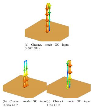
Fig. 9. Characteristic mode currents for a basic folded monopole antenna.
