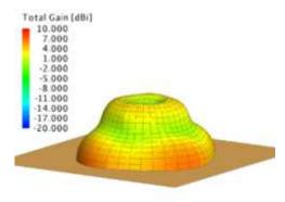
Fig. 19. Radiation pattern of the characteristic mode with an open-circuited input at 1554 MHz (fcp3).
