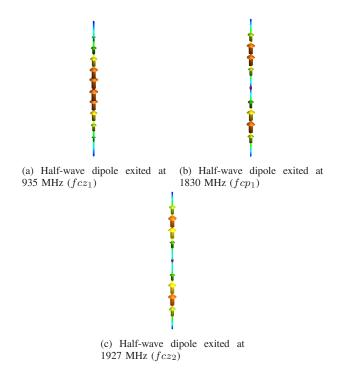
Fig. 6. Currents of the half-Wave dipole exited with a resistive source.
