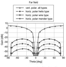
co and cross polar gain (.75 GHz, Phi = 0)
