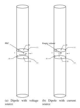
Fig. 4. Half-wave dipole with voltage and current excitation.
