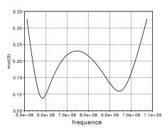
Fig. 22. Magnitude of the reflection coefficient  $(S_{11})$  of the cage antenna for a VSWR<2 bandwidth.
