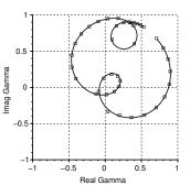
Fig. 13. Real versus imaginary part of the input reflection coefficient (Gamma) of the cage antenna between 300 MHz and 1.8 GHz. The square points correspond to the simulation values. The full line corresponds to the interpolation with the rational fraction.
