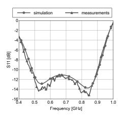
Fig. 28. Measured and Modeled reflection coefficient.
