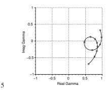
Fig. 8. Real versus imaginary part of the input reflection coefficient of the basic folded monopole antenna between 400 MHz and 1.7 GHz. The square points correspond to the simulation values. The full line corresponds to the interpolation with the rational fraction.
