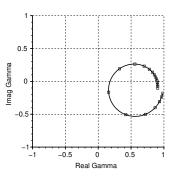
Fig. 1. Real versus imaginary part of the input reflection coefficient of the dipole antenna between 400 MHz and 2 GHz. The square points correspond to the simulation values. The full line corresponds to the interpolation with the rational fraction.
