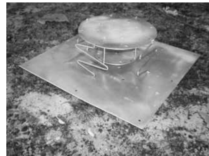
Fig. 27. Picture of the antenna with four meander-line and only a part of the ground plane (The 1x1 m ground plane is not shown).
