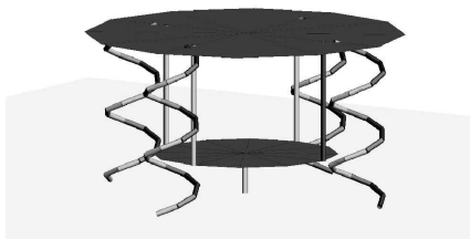
Fig. 23. Four helix wires Antenna. Dimension (see Fig.12) h_1 = 6 cm, h_2 = 1.5 cm, D_1 = 12 cm, D_2 = 7 cm, Wire diameter 2 mm, helix diameter: 10 mm, N_{turn} = 2.5 .
