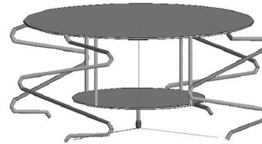
Fig. 26. Realized meander lines Antenna. Dimension (see Fig.12)  $h_1 = 6.16$  cm,  $h_2 = 1.5$  cm,  $D_1 = 12$  cm,  $D_2 = 7$  cm, input wire diameter 1.1 mm, All other wires diameter 1.8 mm, meander-line width: 66 cm, metallic plates thickness .8 mm.
