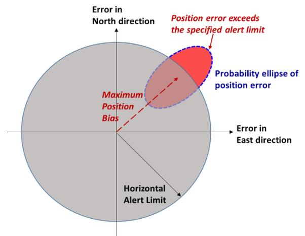
Figure 1 – Position error probability distribution and protection region
