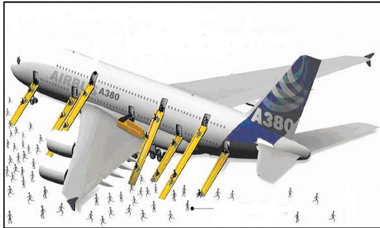
Fig. 1. A380 - 90 seconds Evacuation Demonstrations: 873 occupants(853 Passengers + 20 Crews) [3]
