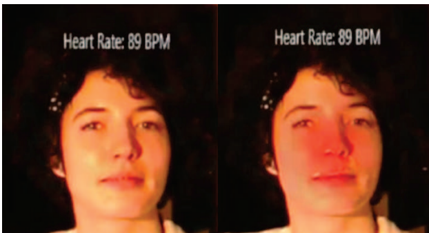
Figure 4: Screenshots of the Cardiolens blood flow augmentation captured during an interaction. The system magnifies minute variations in blood flow captured via the front-facing camera.
