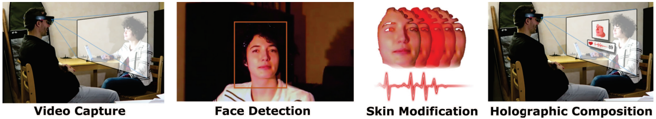
Figure 3: Video transformation pipeline for analyzing the physiological signals of another person. The video is captured and processed to extract the subject’s heart beat from the facial region-of-interest. Then the system magnifies minute variations in blood flow via modifications to the skin pixel intensities. Finally, holograms are anchored to display the magnified blood volume pulse and heart rate information.
