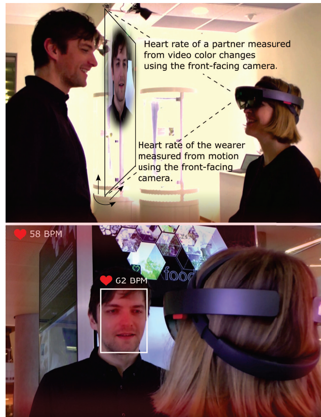
Figure 1: Cardiolens is a mixed reality system that allows simultaneous physiological measurement of multiple people, including the wearer. The physiological signals are visualized in the real-world allowing the wearer to see magnified blood perfusion and vital signs in real-time.
