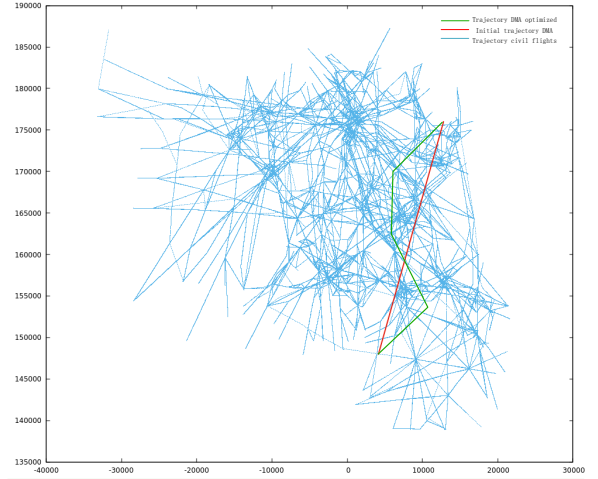
Figure 8 Simulated France traffic consists of 8,836 flights, initial mission trajectory, and optimized mission trajectory.
